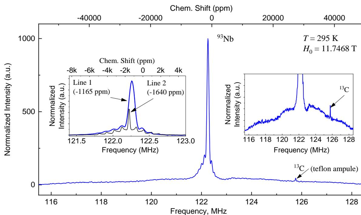
**Figure 3** The  $^{93}\text{Nb}$  NMR spectra for LLZ-Nb obtained at room temperature. Left inset shows an enlarged fragment and the presence of the second spectrum component (black line is simulation). Right inset shows enlarged fragment and the shape of the pedestal and the signal from the polytetrafluoroethylene ampoule
