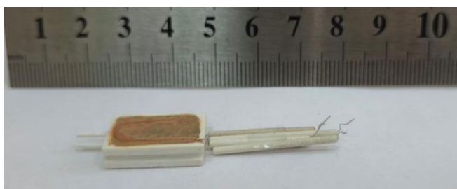
Figure 2 Appearance of the YSZ-YSZ sensor with the intermediate layer and activated Pt electrodes.
