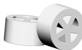
Figure 4 Shape of the pellet of the catalyst guard bed
