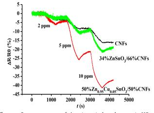
Figure 4 Sensor response of zinc stannate-based sensor to  $NO_2$  (25±1  $^{\circ}C$ ).
