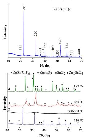
**Figure 1** Diffractograms of the freshly deposited sample (1) and thermolysis products obtained at temperatures 300...500 (2), 650 (3) and 800 (4) (Cu K $\alpha$  radiation).
