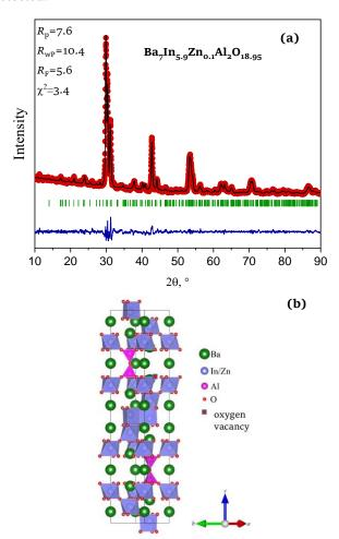
**Figure 1** Rietveld profile fitting of powder X-ray diffraction pattern for the dehydrated  $Ba_7In_{5.9}Zn_{0.1}Al_2O_{18.95}$  sample. The experimental data are given as red circles, the fitted profile as solid black line. The vertical bars indicate the expected positions of the Bragg peaks upon refinement in the space group  $P6_3/mmc$ . The bottom blue line represents the difference between the calculated and experimental data (a). Crystal structures of the investigated sample (b).
