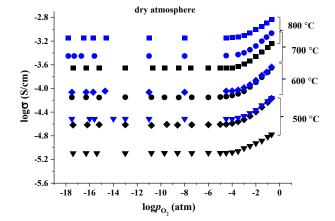
**Figure 6** Dependencies of the conductivity vs oxygen partial pressure at different temperatures for  $Ba_7In_{5.9}Zn_{0.1}Al_2O_{18.95}$  (blue symbols) and  $Ba_7In_6Al_2O_{19}$  (black symbols) in a dry atmosphere.
