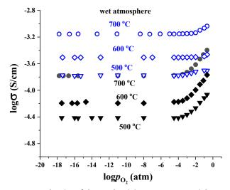
**Figure 9** Dependencies of the conductivity vs oxygen partial pressure at different temperatures for  $Ba_7In_5.9Zn_{0.1}Al_2O_{18.95}$  (blue signs) in comparison with  $Ba_7In_6Al_2O_{19}$  (black signs) in a wet atmosphere.
