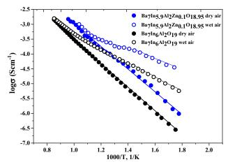
**Figure 5** Comparison of the temperature dependencies of the conductivities of doped  $Ba_7In_{5.9}Zn_{0.1}Al_2O_{18.95}$  and undoped  $Ba_7In_6Al_2O_{19}$  samples in dry (pH<sub>2</sub>O = 3.5·10<sup>-5</sup> atm, filled signs) and wet (pH<sub>2</sub>O = 1.93·10<sup>-2</sup> atm, open signs) air.
