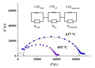
Figure 3 Impedance spectra of  $Ba_7In_{5.9}Zn_{0.1}Al_2O_{18.95}$  at different temperatures in dry air  $(pH_2O=3.5\cdot10^{-5}$  atm).
