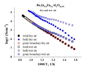
**Figure 4** Temperature dependencies of the bulk, grain-boundary and total conductivities for  $Ba_7In_{5.9}Zn_{0.1}Al_2O_{18.95}$  in dry  $(pH_2O=3.5\cdot10^{-5}$  atm, filled signs) and wet  $(pH_2O=1.93\cdot10^{-2}$  atm, open signs) air.
