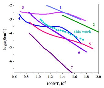
**Figure 10** Comparison of the temperature dependencies of the conductivities in wet air for  $Ba_7Nb_{3.8}Mo_{1.2}O_{20.1}$  (1) [46],  $Ba_7Nb_4MoO_{20}$  (2) [20],  $Ba_5Er_2Al_2ZrO_{13}$  (3) [24],  $Ba_5Lu_2Al_2ZrO_{13}$  (4) [24],  $Ba_5In_2Al_2ZrO_{13}$  (5) [34],  $BaLaIn_{0.5}Y_{0.5}O_4$  (6) [47],  $BaLaInO_4$  (7) [47] and  $Ba_7In_{5.9}Zn_{0.1}Al_2O_{18.95}$  (this work, circles).
