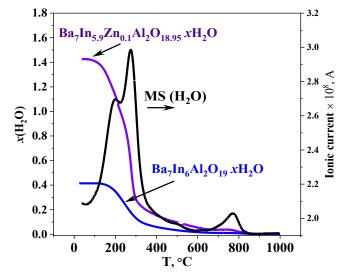
Figure 2 TG and MS(H<sub>2</sub>O) curves for Ba<sub>7</sub>In<sub>5.9</sub>Zn<sub>0.1</sub>Al<sub>2</sub>O<sub>18.95</sub>, and the TG curve for  $Ba_7In_6Al_2O_{19}$ .
