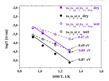
**Figure 7** Temperature dependencies of the ionic conductivities of  $Ba_7In_{5.9}Zn_{0.1}Al_2O_{18.95}$  in comparison with  $Ba_7In_6Al_2O_{19}$  for dry  $(pH_2O=3.5\cdot10^{-5}$  atm, filled signs) and wet  $(pH_2O=1.93\cdot10^{-2}$  atm, open signs) atmospheres.
