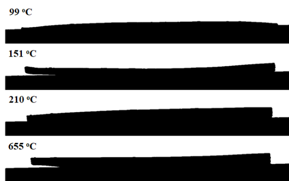
Figure 3 Optical micrographs of LLZ film during heating (2 °C min -1 ).
