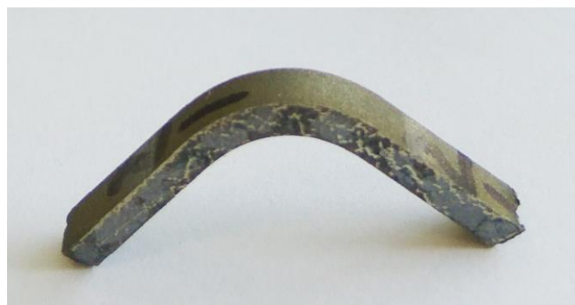
Figure 7 The sample sintered for 0.5 min bending tests when applying the force perpendicular to the layers.
