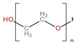
**Figure 1** The structure of the polyethylene glycol molecule and its representation in the Martini force field 2.2. SNa-SH<sub>2</sub>-...-SH<sub>2</sub>-SNa; SNa - terminal OH group; SH<sub>2</sub> is a polyethylene glycol monomer.
