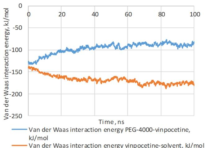
**Figure 4** Van der Waals interaction energy of vincopetine with PEG-4000 and solvent in terms of one molecule of vincopetine at a ratio of vincopetine and PEG-4000 1:2 by weight.
