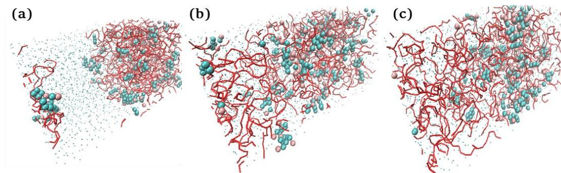
**Figure 6** Simulation of the molecular dynamics of the release of vincopetine from an alloy with polyethylene glycol-4000 1:5 by weight into water. Time is 0 ns (a), 40 ns (b), 100 ns (c).
