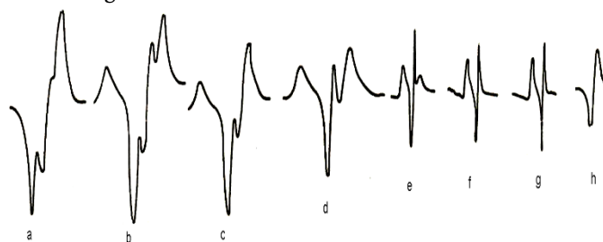
Fig. 8 Annealing of paramagnetic centers on gamma-irradiated BeO. ( D_\gamma = 18.6 mrad). a - T = 20 , b - 60, c - 120, d - 170, e - 240, f - 360, g - 460, h - 480 °C
